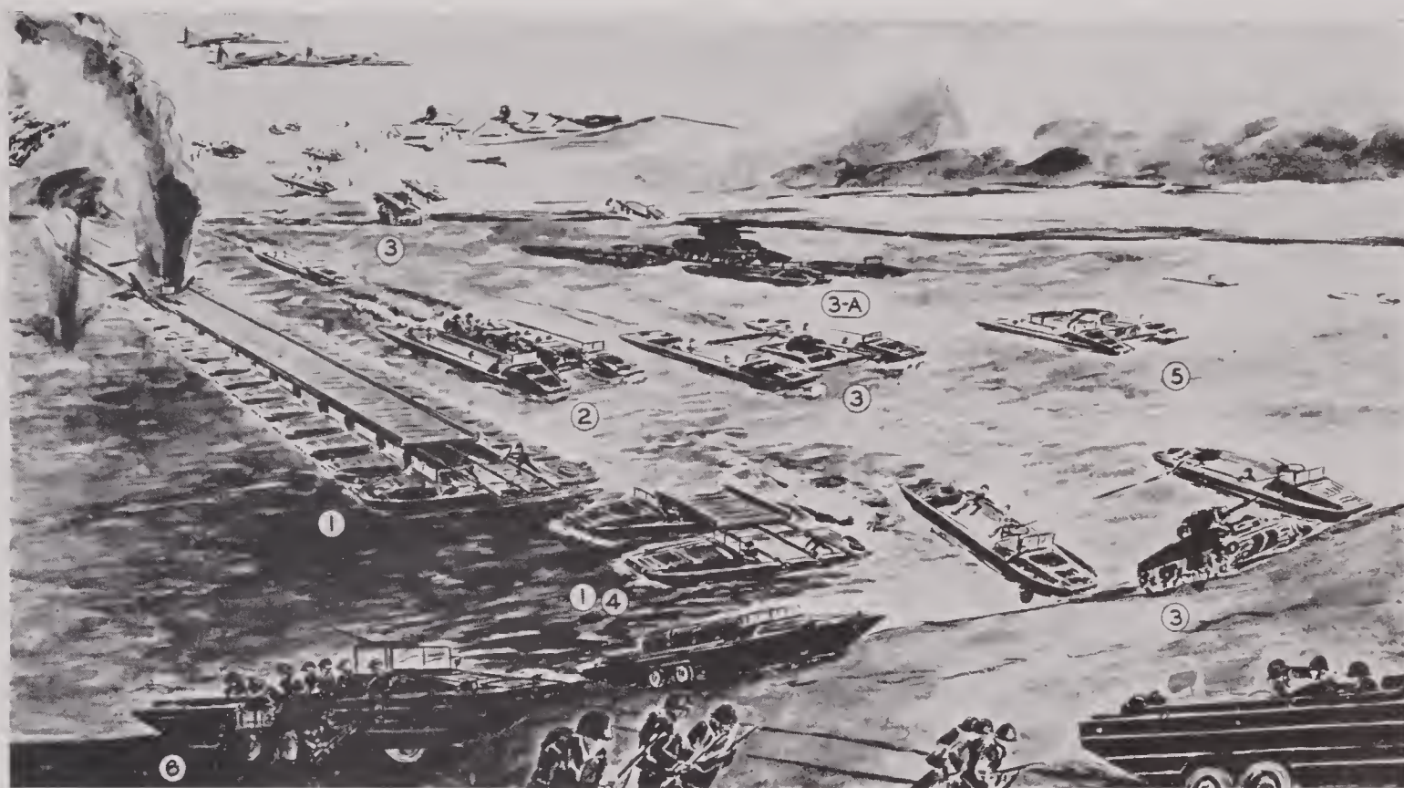
FIGURE 46. Artist's conception of some proposed uses of DUKW: (1) ponton bridge, (2) vehicle ferry, (3) tank wet ferry, (3A) tank dry ferry, (4) light freight carrier, (5) heavy freight carrier, and (6) troop carrier.
